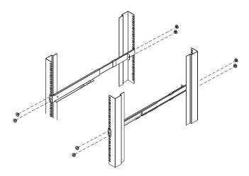
4. Slide the switch onto the support flanges. Use the screws supplied with this package to loosely attach the front of the switch to the front of the rack (only tighten the screws part way).
